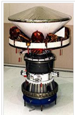
Mars Pathfinder during final assembly showing the aeroshell, cruise ring and solid rocket motor
