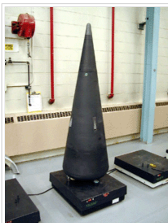
Mk-12A RV retrofitted with hafnium diboride strakes for a NASA research project (Sharp-B2)
