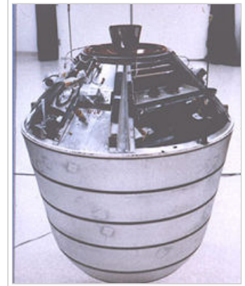
"Discoverer" type reconnaissance satellite film Recovery Vehicle (RV)
