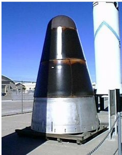
Mk-6 RV, Cold War weapon and ancestor to most of NASA's entry vehicles
