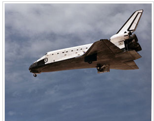
LI-900 is a rigid black tile on the Space Shuttle. (Shuttle shown is Atlantis.)
