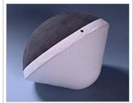
Deep Space 2 aeroshell, a classic 45° sphere-cone with spherical section afterbody enabling aerodynamic stability from atmospheric entry to surface impact
